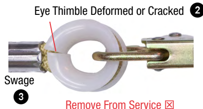
Fig.9 Lanyard Inspection 1
