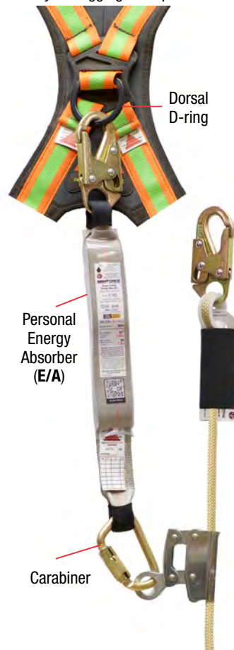
Fig.2 Full Body Harness Lanyard Rigging Example
