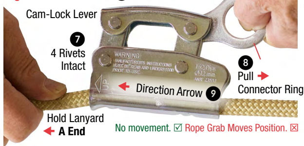
Fig.7a Cam-Lock Test 7
