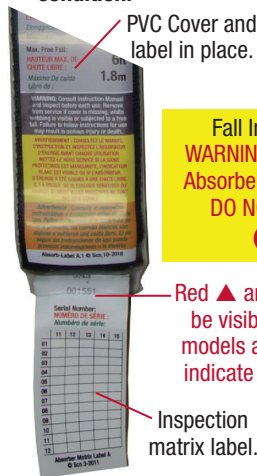
Fig.12 Absorber serviceable condition.
