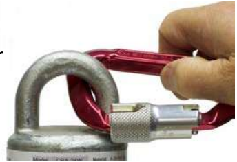
Fig.2.2 Non-compatibility. Do not attach two connectors to a loop top.
