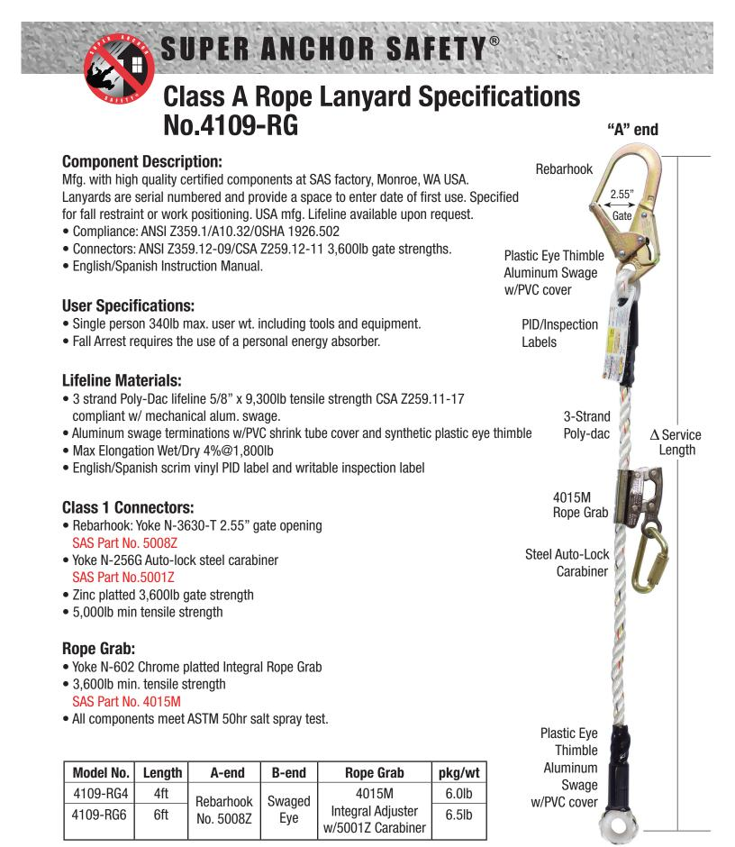
$\Delta$  Service Length measured from connector ends
