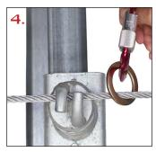
Rotate the **O**-Ring away from the loops completing the Pass-Thru. Reverse the procedure to pass back thru.
