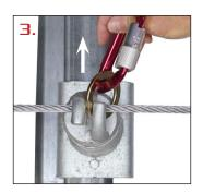
Pull O-Ring away from the loops and apply downward pressure to the cable at the same time.
