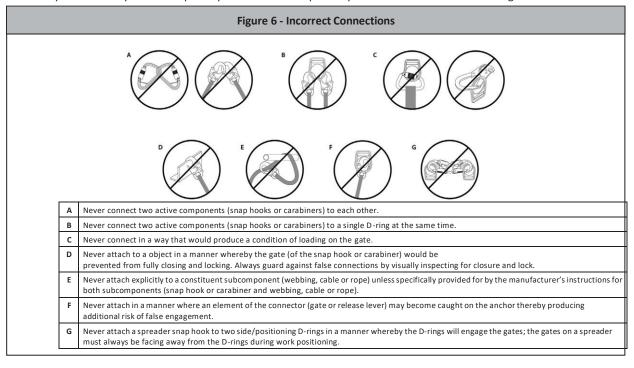
**3.4 Connectors:** Only use self-locking snap hooks, rebar hooks, and carabiners with this equipment. Only use connectors that are suitable to each application. Ensure all connections are compatible in size, shape and strength. Do not use equipment that is not compatible. Visually ensure all connectors close and lock completely. Connectors (snap hooks, rebar hooks, and carabiners) are designed for use only as specified in this manual.
