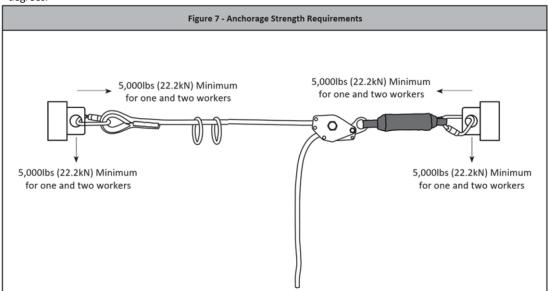
**Step 1:** Determine the location of the end anchorages and, in accordance with Section 3.2, evaluate their strength. Determine the span length of the system and determine the minimum required clearance for safe use in accordance with Section 2.7.
