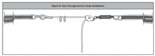
Step 3: Secure the HLL system to the anchorage connectors with the provided end attachment carabiners.
