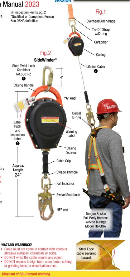
Units removed from service must be disposed of in a way that prevents further use and prevents the possibility of someone dismantling the SRL. Due to the acute danger posed by the recoil spring, it is recommended to return non-serviceable units to the SAS factory for safe disposal.
