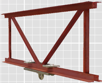
Steel Web Truss
