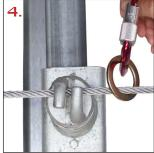
Pull **O**-Ring away from the loops and apply downward pressure to the cable at the same time.
