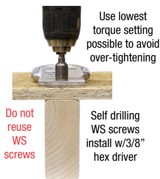
Fig.5 WS Screw Installation
