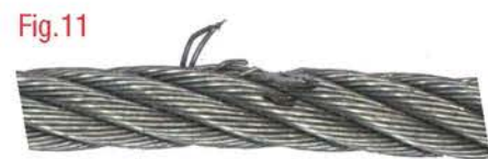
Do not use lanyards with burrs, cuts or gouges.
