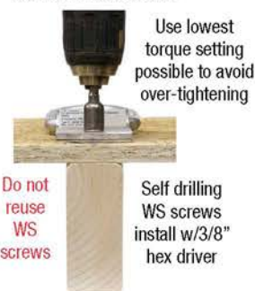
WS Screw Installation
