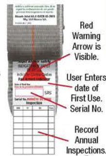
Fig.12b Serviceable Condition. Backer Webbing Covers the Fall Indicator
