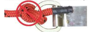
Fig. 20d DO NOT Tie a Lifeline to a Anchorage Point Attach Lifeline A-end w/class 1 connector only.
