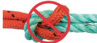
Fig. 20c DO NOT Tie Lifelines Together
