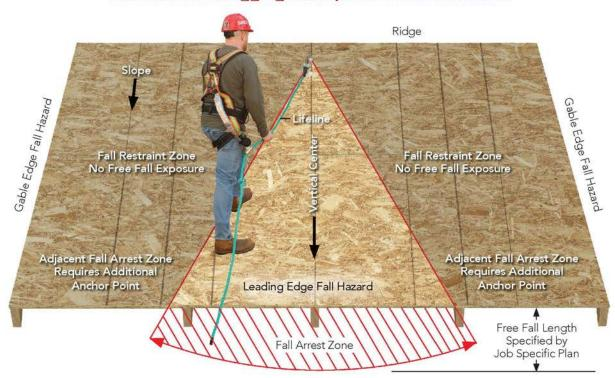
Note: SRL's are not designed to restrain a worker from traveling over a leading edge. For that reason a Class 2 SRL-LE can be used in lieu of a lifeline system in fall arrest.
