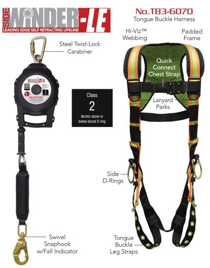
OSHA requires that SRL's anchored at or below a full body harness dorsal D-ring, are rated for leading edge Class 2. This would apply to roofers, roof loaders, framers, truss stackers, interior and exterior work, and leading edge hazard exposure. Any work performed where an overhead anchorage is not available.
