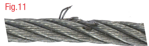
Do not use lanyards with burs, cuts or gouges.
